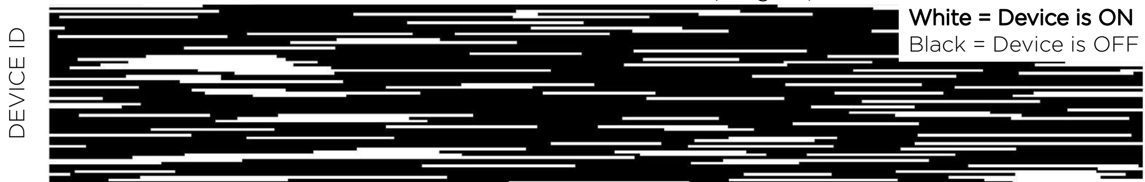
CONVENTIONAL THERMOSTAT (long on/off times)
