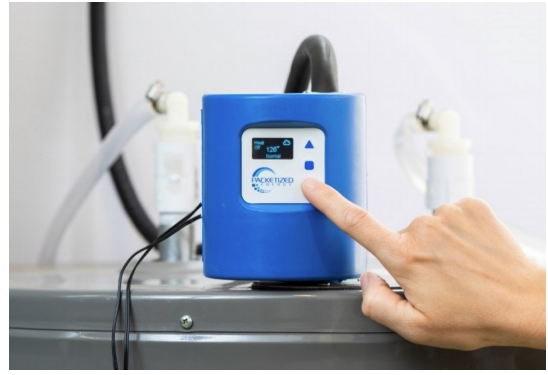
Fig. 2. The water heater management device used in this work, known as the Mello™ smart thermostat for water heaters. Two temperature sensors allow the device to measure the water/tank temperature near the tank’s upper and lower thermostats. Users can adjust the temperature set point (the middle of the flexible range) using the buttons on the device or through a phone app.
